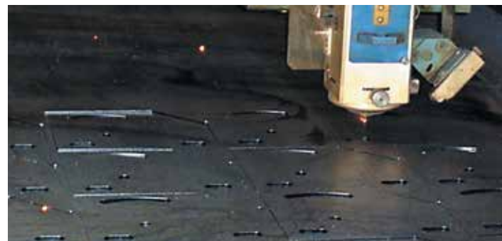
Above: Janco Industries uses laser to produce structures and components for its agricultural, construction and food processing equipment customers, working in various mild and stainless steel plate.
