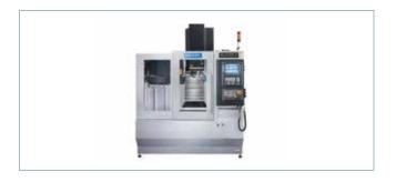
This Sharp SVL-2416 is equipped with the SINUMERIK 828D CNC — the ideal control for compact-class machine tools.
